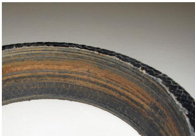
Figure 3. Packing failure from over compression and insufficient flush.
