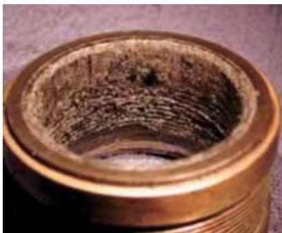
Figure 1. Calcium carbonate build up at the atmospheric side of a seal face
