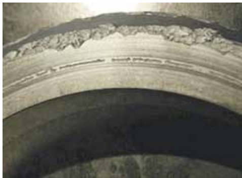
Figure 2. Silicon carbide mechanical seal face damaged by electro-corrosion
