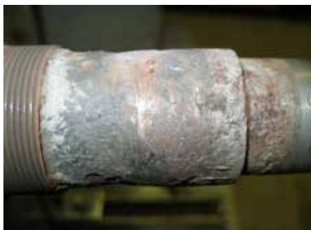
Image 1 (left): Corroded stem. Image 2 (right): Corroded pump shaft (Images courtesy of A.W. Chesterton/Fluid Sealing Association)
