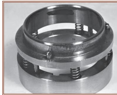
**Figure 1. Seal with excessive wear on drive pins, dents, and slot**
