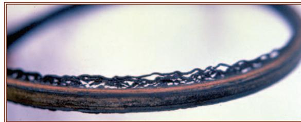
**Figure 2. O-ring exhibiting extrusion.**
