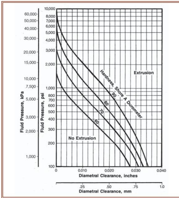
Figure 3. Allowable clearances for O-ring secondary seals.
