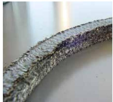
(left to right) Image 1. Extrusion of the seal material Image 2. Charred packing Image 3. Abraded packing (Images courtesy of the author)
