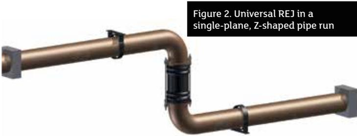
Figure 2. Universal REJ in a single-plane, Z-shaped pipe run
