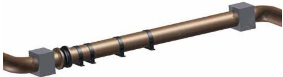
Figure 1. Unrestrained REJ in straight-anchored and well-guided pipe run
