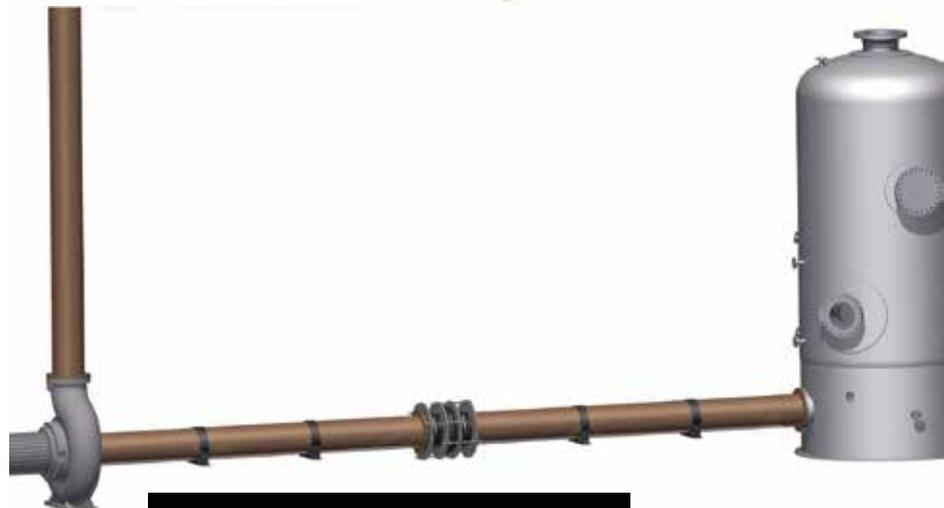
Figure 5. In-line pressure-balanced REJ in straight pipe run with load limitations
