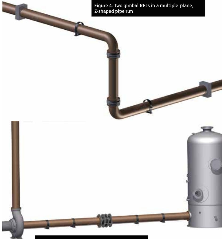
Figure 4. Two gimbal REJs in a multiple-plane, Z-shaped pipe run
