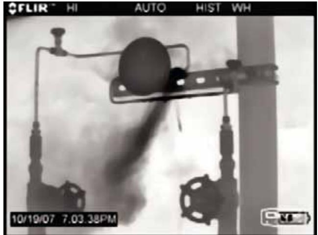
VOC leak detected with FLIR camera (Courtesy of FLIR Systems, Inc.)
