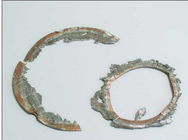
Figure 56: Gasket Chemical Attack
