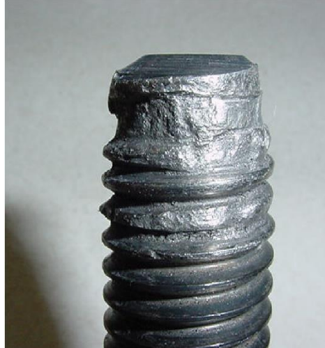
Figure 43: Galled Stainless Steel Bolt
