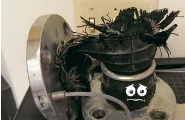
IMAGE 4: Failed expansion joint
