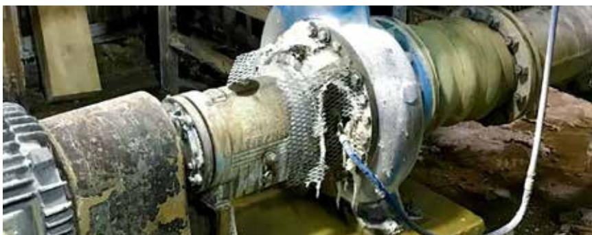
IMAGE 1: A damaged shaft leads to reduced sealing quality (Image courtesy of FSA)
