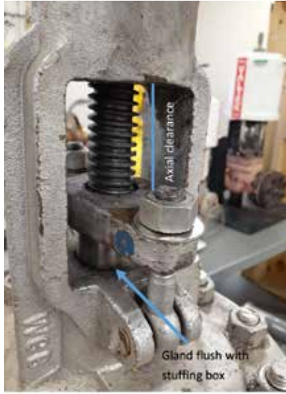
IMAGE 4: Conditions for measuring axial clearance: packing installed, gland out of stuffing box
