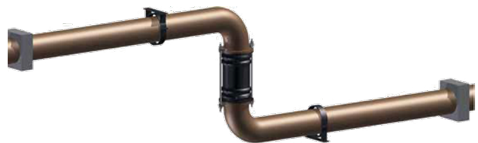
Figure 5B: Typical Layout Utilizing Expansion Joints and the Proper Use of Anchors in Branch Locations
