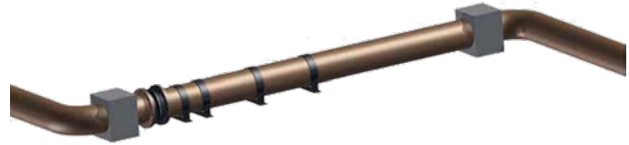
Figure 5A: Typical Piping Layout Utilizing Expansion Joints When Equipment and Piping are Properly Anchored
