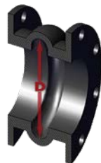
Figure 3. Thrust forces on expansion joint.
