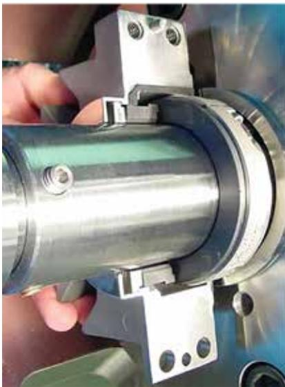
IMAGE 4: Split seal during installation (Image courtesy of Flowserve)
