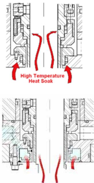
IMAGE 2: A properly designed cooling spool can prevent excessive temperatures that can result in damage.
