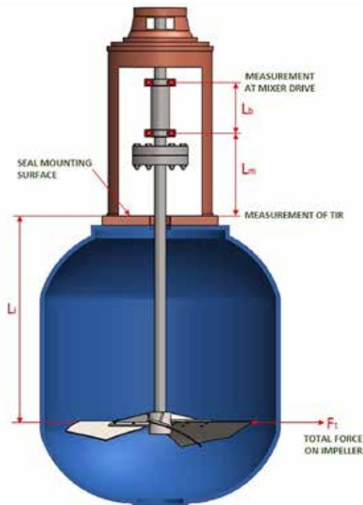
IMAGE 1: The deflection can be calculated if key attributes of the shaft and shaft loading are known. (Images courtesy of FSA)
