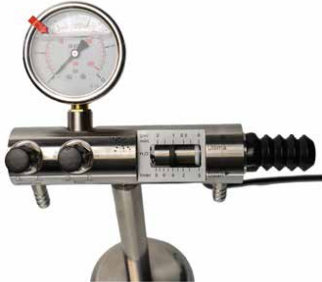
IMAGE 1: Flow meter with pressure gauge and control valves (Images courtesy of Fluid Sealing Association)
