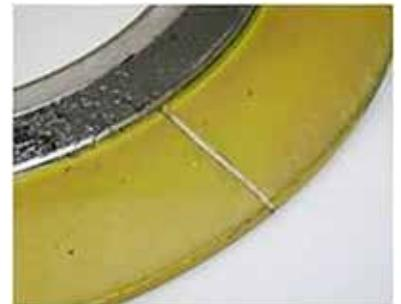
IMAGE 4: Grooves in four positions on outer ring of gasket prior to testing
