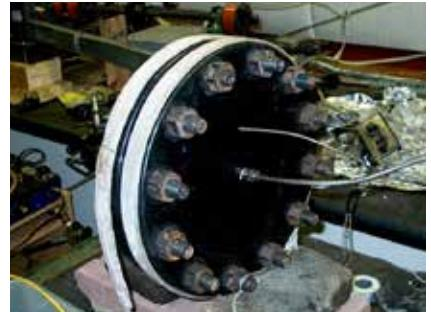
IMAGE 3: A 6-inch class 300 flange assembly heated with wrap heaters
