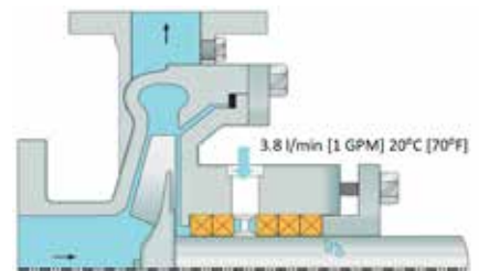
IMAGE 1: Packed pump with dynamic shaft/sleeve sealing surface requiring replacement over time (Images courtesy of Fluid Sealing Association)
