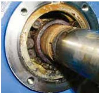
IMAGE 1: Pump bearing failure (Images courtesy of A.W. Chesterton Company)
