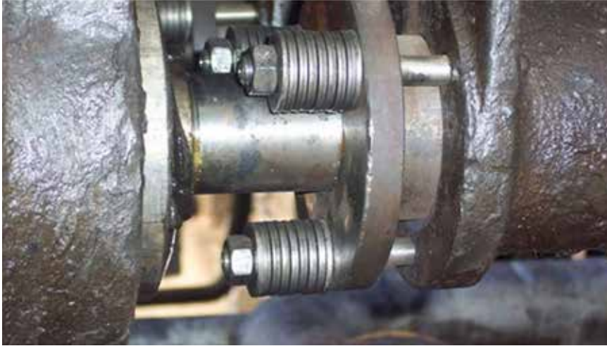
IMAGE 4: Gland nuts can help store elastic energy when gland load is lost due to consolidation
