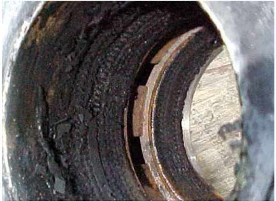
IMAGE 1: Compression packing that is compromised due to wear (Images courtesy of the author)
