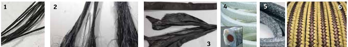
IMAGE 1: Continuous filament graphite-coated carbon yarn (Images courtesy of the author). IMAGE 2: Continuous filament graphite-coated PTFE yarn. IMAGE 3: Extruded ePTFE tape yarn coated with graphite. IMAGE 4: Interbraided rubber core packing. IMAGE 5: Square braid packing. IMAGE 6: Interbraided graphite-coated PTFE with Kevlar packing
