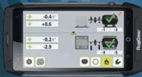
Tackle shaft misalignment efficiently with the AT-100, a horizontal alignment tool designed for novices and experts alike.
