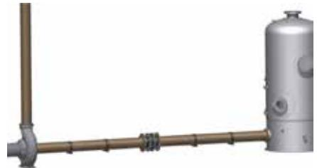
IMAGE 5: In-line pressure-balanced restrained style, in straight pipe section with load limitations
