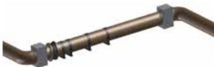
IMAGE 1: Unrestrained style, in a straight well-anchored and well-guided pipe section (Images courtesy of FSA)
