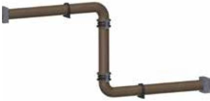
IMAGE 3: Hinge restrained style, in a single plane Z-shaped pipe section
